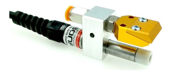
Compressed-air ionizing nozzles have a double function, cleaning the surface of interest and eliminate existing electrostatic charges. Ionizing nozzles are employed where installation conditions are critical, especially in confined spaces. Our ionizing nozzles can have multiple configurations and can be connected in series even in circular shape according to customer's needs.
