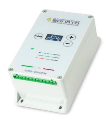
**EASY CHARGE** charging generator creates an adjustable high voltage between 0 to 20 KV and an also adjustable current between 0 and 1,0 mA. Its controls are very intuitive and thus easy to be used by the operator also thanks to the oled display, where you can read both voltage, istantaneous current and working mode; moreover, it can be remotely controlled by means of the remote control analogical function. It can have positive or negative charge on request and up to 2 exits.
