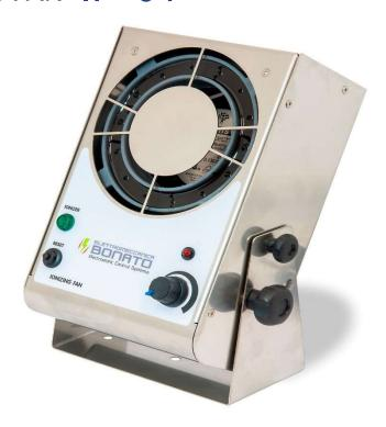
The IF-01 ionizing fan has been designed to break down antistatic charges very quickly and bring the balance to +/- 3V.
